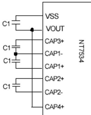
4x step-up voltage circuit (C1 = 1.0 ~ 4.7 uF)
