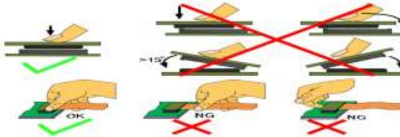
5. Precaution for soldering the LCM
