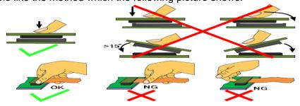
5. Precaution for soldering the LCM
