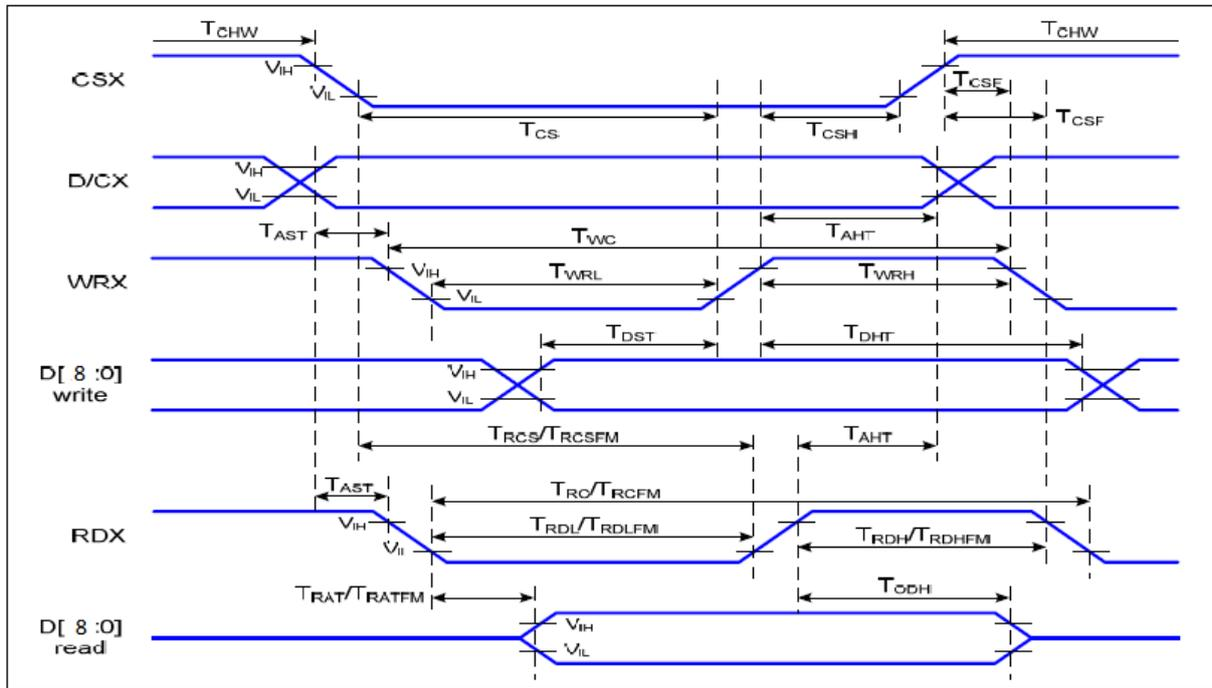
VDDI=1.65 to 3.3V, VDD=2.4 to 3.3V, AGND=DGND=0V, Ta= -30 to 70 °C
