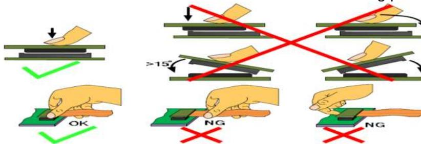
5. Precaution for soldering the LCM
