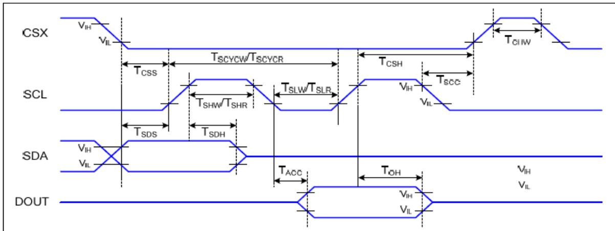
VDDI=1.65 to 3.3V, VDD=2.4 to 3.3V, AGND=DGND=0V, Ta=-30 to 70 °C
