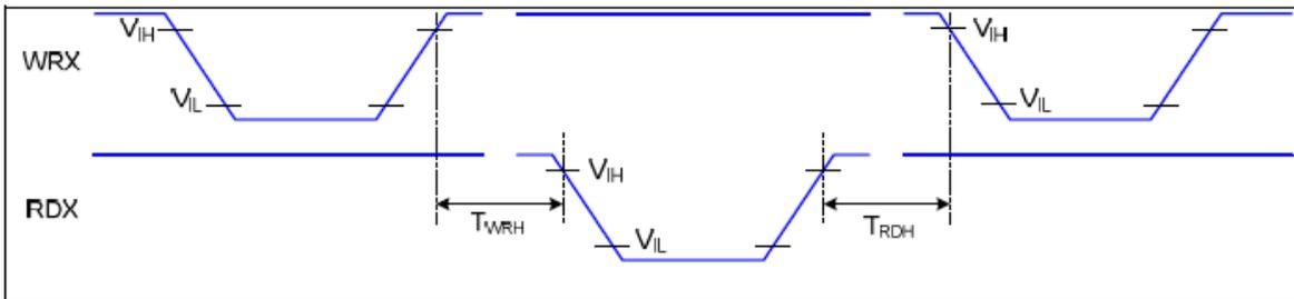
Figure Write-to-Read and Read-to-Write Timing
