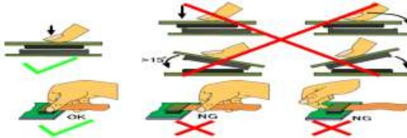
**5. Precaution for soldering the LCM**
