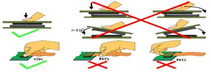
5. Precaution for soldering the LCM
