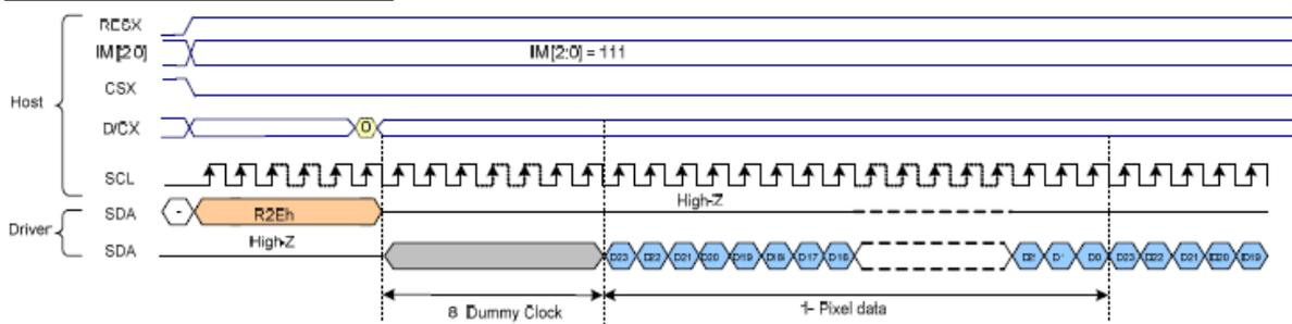
Figure 108: 4-Line SPI Mode Read Data
