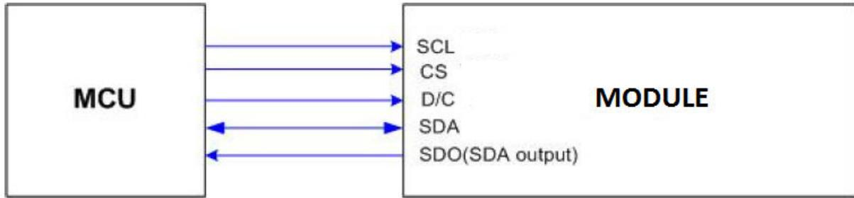
The 4-line/8-bit serial bus can be used by setting external pin IM [2:0] as 111.
