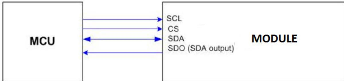
The 3-line/9-bit serial bus can be used by setting external pin IM [2:0] as 101.
