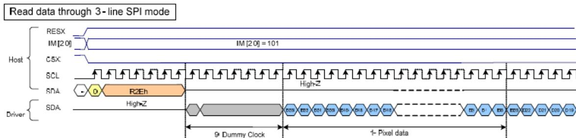
Figure 104: 3-Line SPI Mode Read Data
