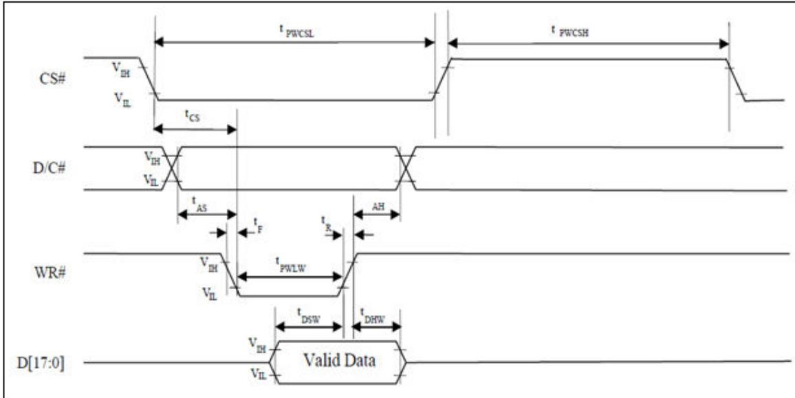
Figure 8-1: Parallel 8080-series Interface Timing Diagram (Write Cycle)
