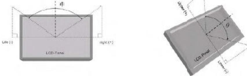
Fig.6-2 Definition of Viewing Angle
