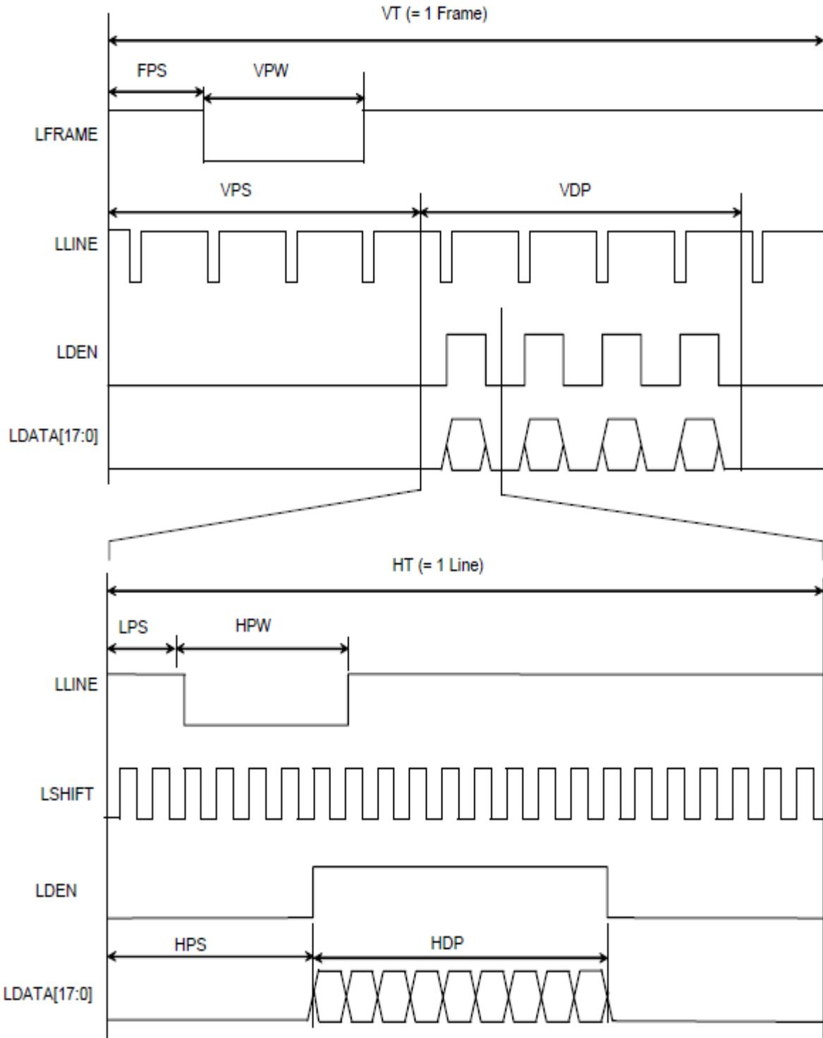
Figure 8-3: General TFT Panel Timing
