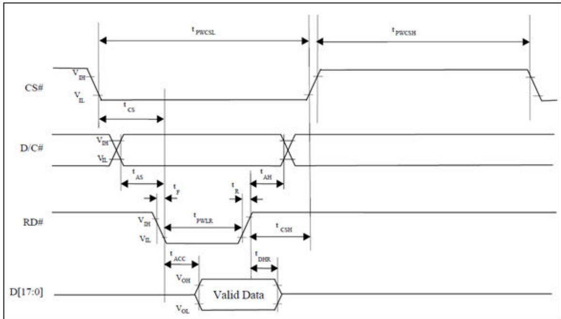
Figure 8-2: Parallel 8080-series Interface Timing Diagram (Read Cycle)
