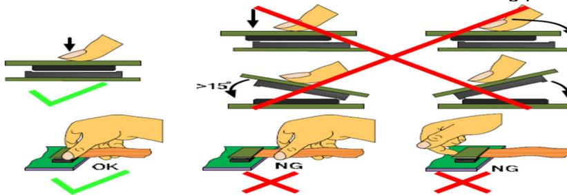
**5. Precaution for soldering the LCM**
