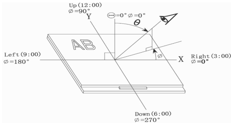
Note 4: Definition of contrast ratio. (Test LCD using DMS501)
