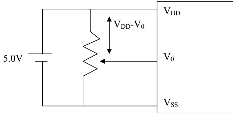
Where  $V_{DD}-V_0 = \text{LCD Driving voltage}$
