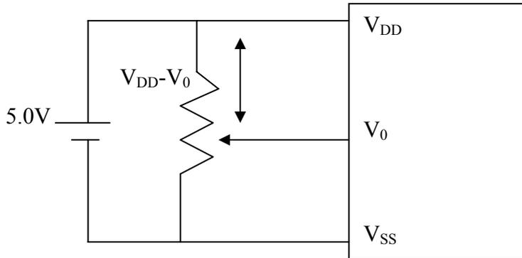
Where  $V_{DD}-V_0$  = LCD Driving voltage
