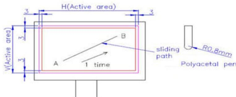
Operation force: 120g max (tip R0.8mm Polyacetal pen operation and R8mm silicon rubber, interval 2mm within Active area.
