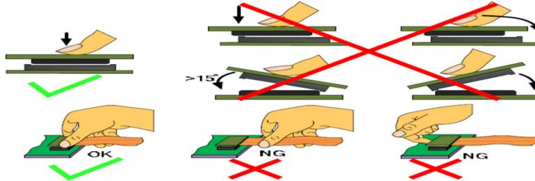
**5. Precaution for soldering the LCM**
