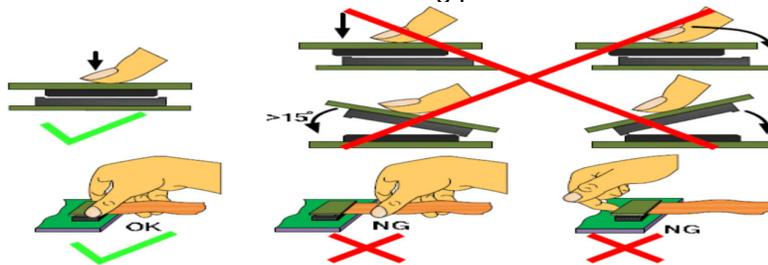
5. Precaution for soldering the LCM
